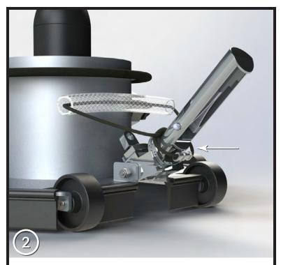
Make sure grommet on Portability Kit handle slides under lip protruding from under swivel handle, securing into place.
